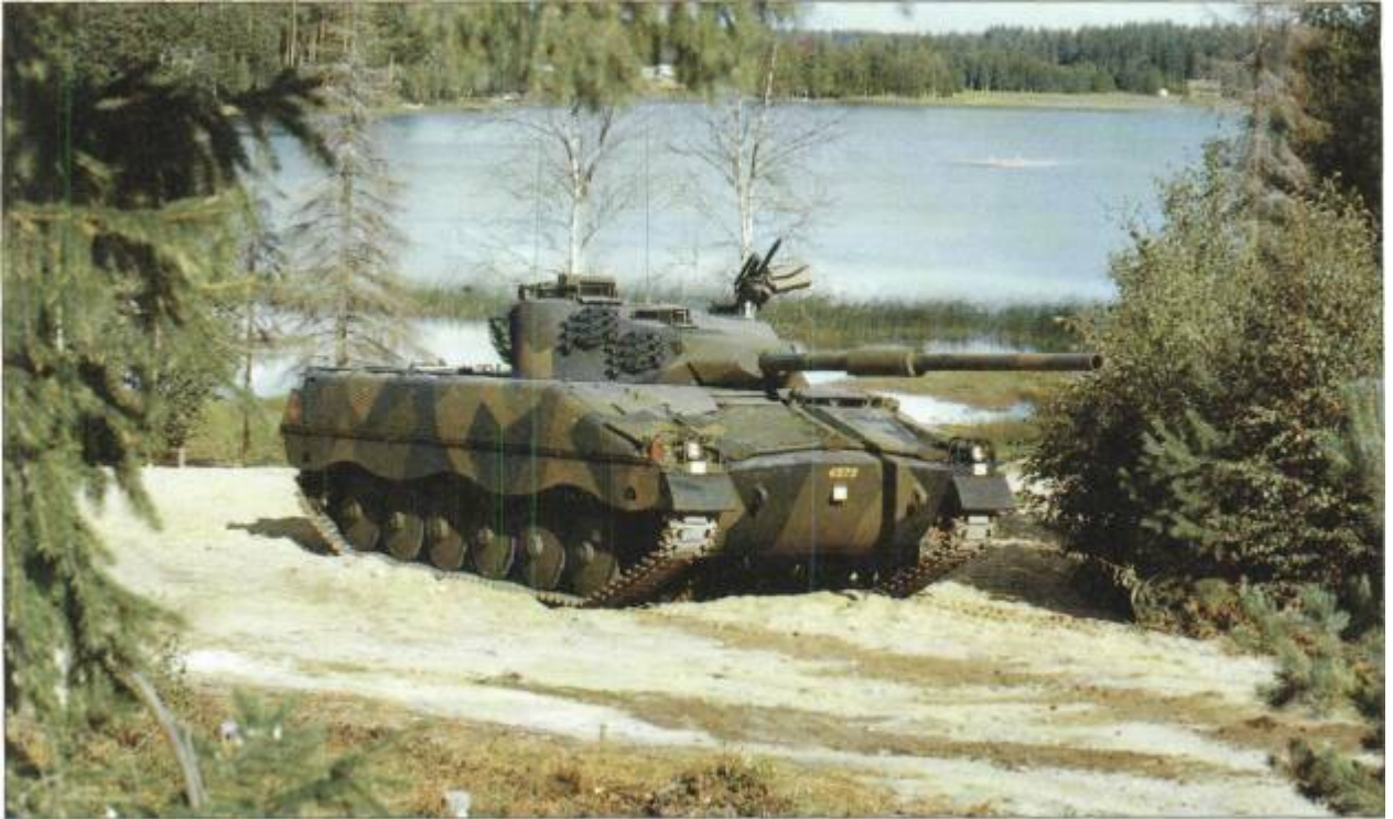
Above: Ikv-91 with trim vane on glacis plate
