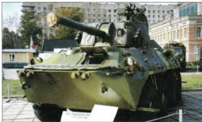
Right: 120mm 2S23 self-propelled gun/mortar system with thermal screens (Christopher F Foss)
