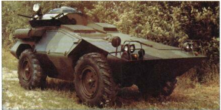
Top right: Commando Scout with 1m turret and twin 7.62mm MG
