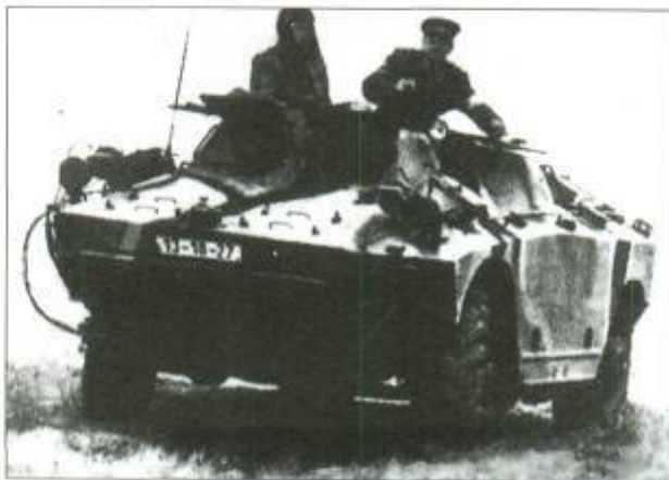
Above right: FUG (4x4) radiological-chemical reconnaissance vehicle with trim vane erected
