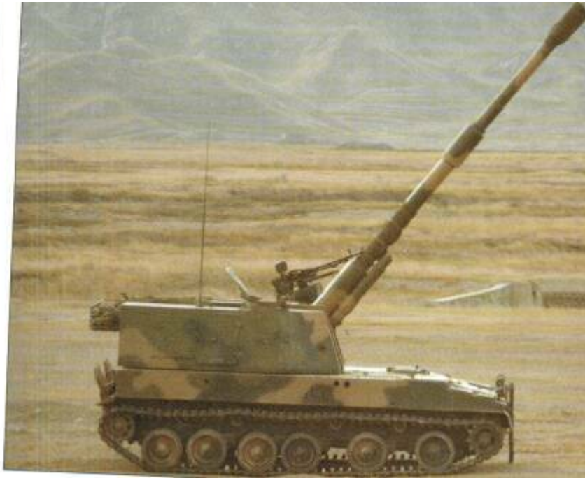
NORINCO 155mm PZL45 self-propelled gun
