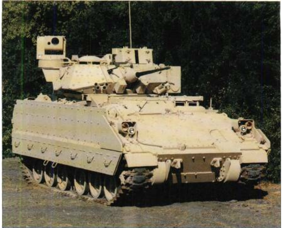
Above: Bradley A3 with applique armour and Commanders Independent Viewer
