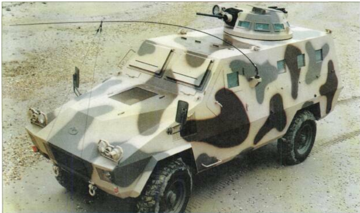
Above: ACMAT VBL light armoured car with one-man turret armed with 12.7mm M2 HB and 7.62mm MGs
