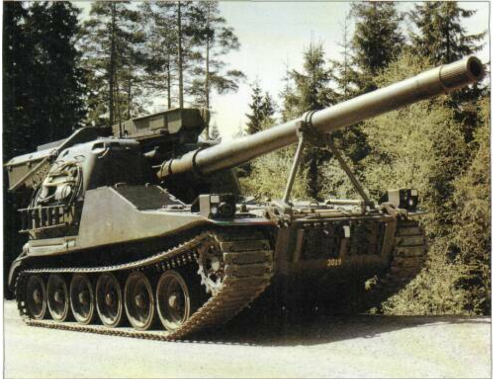
Right: 155mm Bandkanon 1A in travelling configuration
