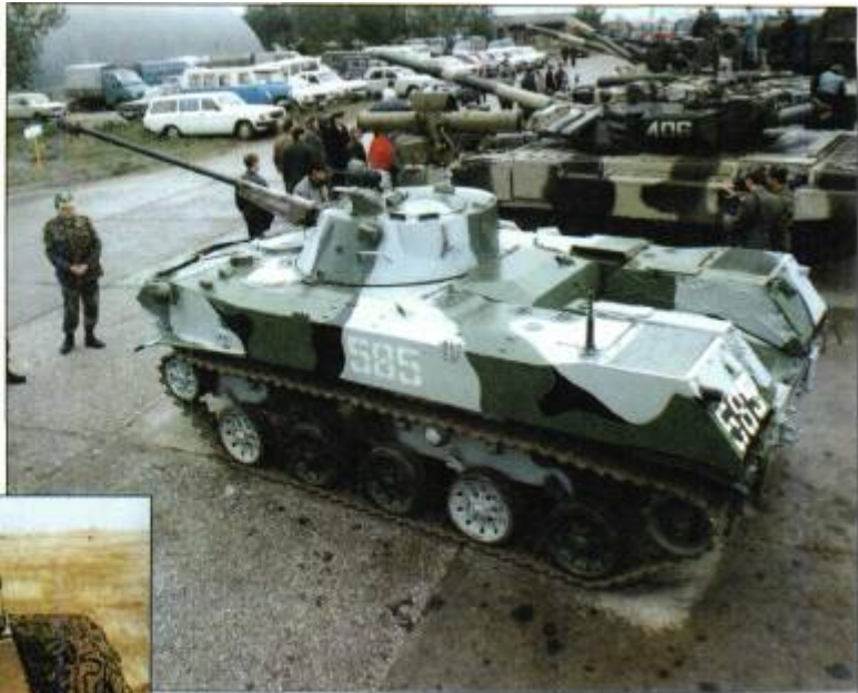
Above: BMD-2 which has new turret armed with 30mm cannon (Steven Zaloga)
