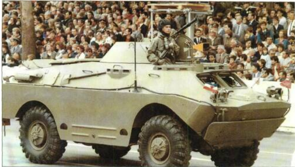
Above: BRDM-2 with commander's and driver's hatches open (Richard Strickland)
