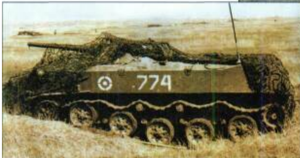
Above: BMD-2 which has new turret armed with 30mm cannon (Steven Zaloga)
